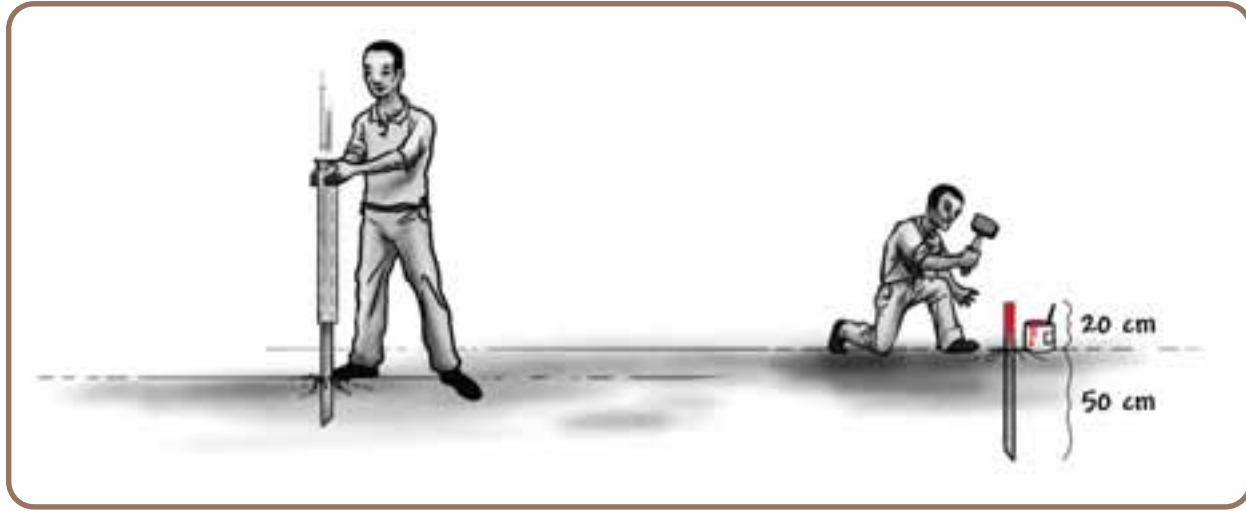
Illustration 73: Marking fixed observation points by driving a painted metal post into the ground
